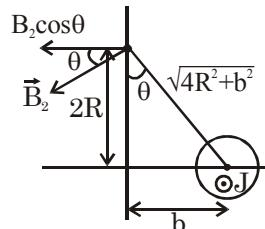
Horizontal component of magnetic field due to smaller wire  $B_{2x}$
