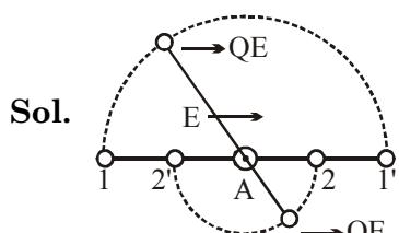
Position of maximum velocity is 1' and 2' for the balls as it is minimum potential energy position
