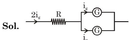
$$V_T = 2i_g R = i_g \times R_g \quad [R_g = R]$$
