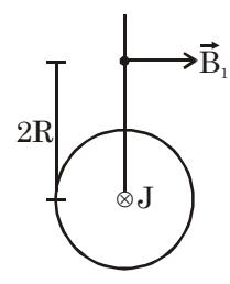
$$B_1 \text{ due to total wire at } y = 2R \text{ is } = \frac{\mu_0 i}{2\pi(2R)} \hat{i}$$
