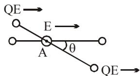
For small angular displacement  $\theta$  from equilibrium position restoring torque
